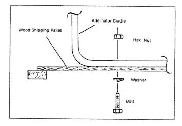
1. The alternator is bolted to a wood shipping pallet. The cardboard is then set into position and retained with straps. Location of alternator and wheel kit in shipping carton is shown above. To remove carton, cut the straps and lift cardboard carton straight up and off pallet.
